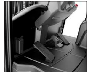
Dual pedal system - forward and reverse.
