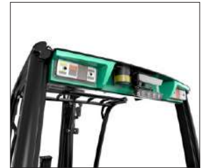
LED working lights, 2 front and 1 rear.
