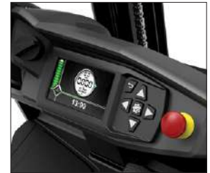
Multifunctional colour display (hourmeter, BDI etc.)
